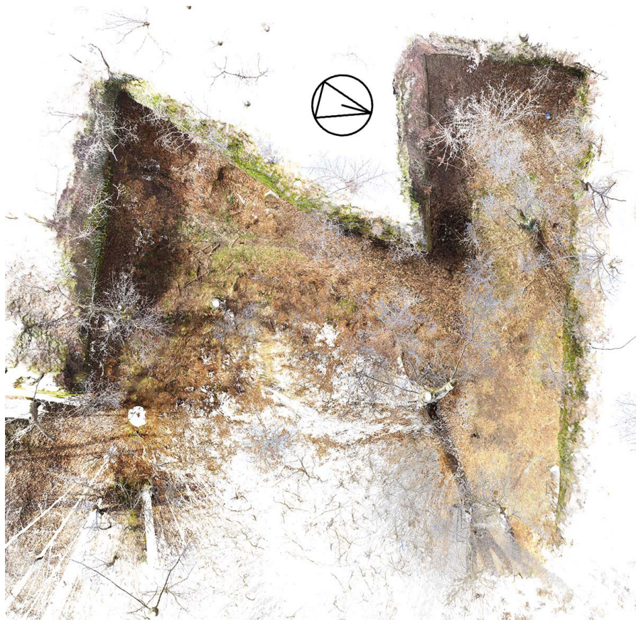
Figure 4. Point cloud overview of the 1225 m 2 area of the abandoned quarry; the point cloud could serve as a basis for a ground floor plan and as a general 3D documentation.
