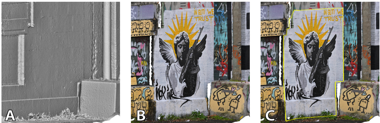
Figure 22. AUTOGRAF can compute a 3D surface mesh (A) with texture (B) from the series of overlapping photos acquired per graffito. On this textured mesh, the GRAPHIS image polygon can be projected (C) to yield a 3D closed polyline whose vertices have real-world 3D coordinates.
