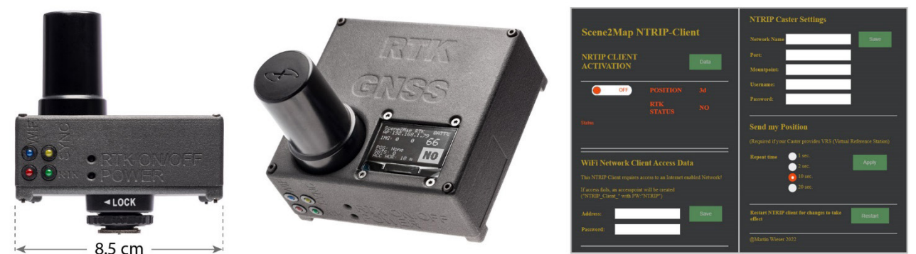
Figure 12. The new RTK-enabled GNSS logging device (left and middle) with the interface controlling its settings (right).
